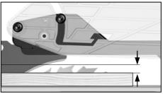
Adjust the cutting depth to the thickness of the workpiece. The sawtooth should come out of the workpiece less than a full tooth height.
