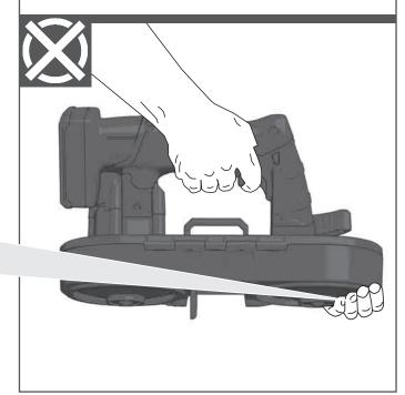
Do not place hand(s) on or around the guard / blade whilst tool has a battery pack connected
