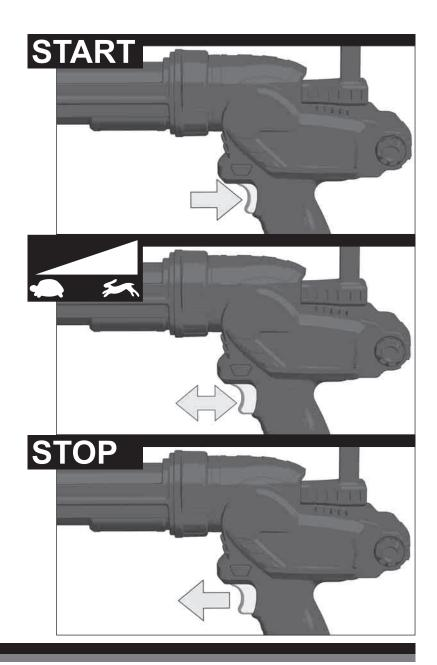
When the trigger is released, the motor will run for a short time to release the rod. This prevents a drip. When a tube is emptied, the motor will run for a short time to release the rod.
