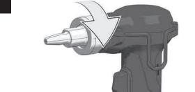
When using Uponor Standard expander heads extra grease needs to be applied in the interface between the tool and the expander head.
