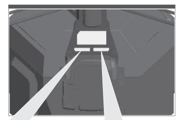
Continuous red: Charging Continuous green: Charging is complete Flashing red: Battery is too hot/cold Flashing red/green: Damaged or faulty battery pack
