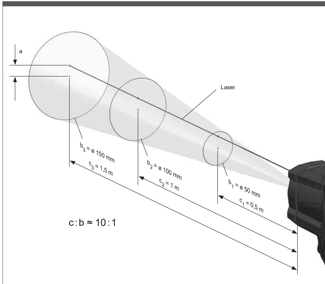
a - Distance laser point to center of spot temperature area (19 mm)
