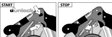
For safety reasons this power tool is fitted with a switch lock and the 0n-/Off switch cannot be locked in the "0n" position.
