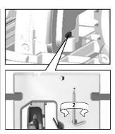
If a correction of the  $90^\circ$  angle of the guide-plate to the saw blade is necessary, use the correction screw.
