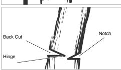
WARNING! Never cut through to the notch when making a backcut. The hinge controls the fall of the tree, this is the section of wood between the notch and backcut. Never position yourself directly behind the trunk of a falling tree. There is a risk that the trunk may split and come back towards the operator.
