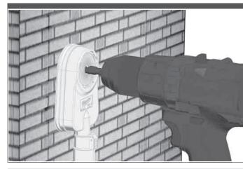
Connect the machine to a suitable dust extractor.
