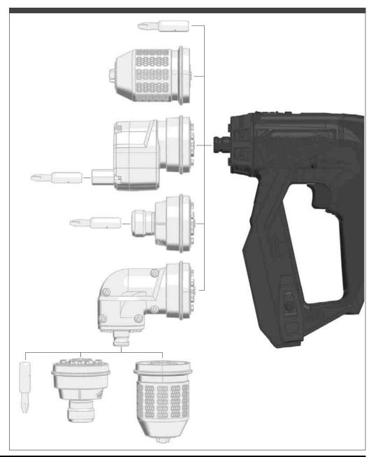
The overview shows a selection of different application heads to this Milwaukee powerbase. Depending on the equipment package you have purchased various application heads. Other application heads and powerbases can be purchased separately. Use only the imaged application combinations of application heads.
