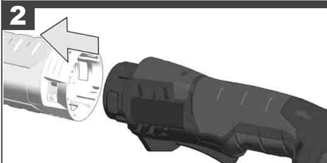
The powerbase may be operated only with a mounted application head. There are three possible positions (application head only as an example).
