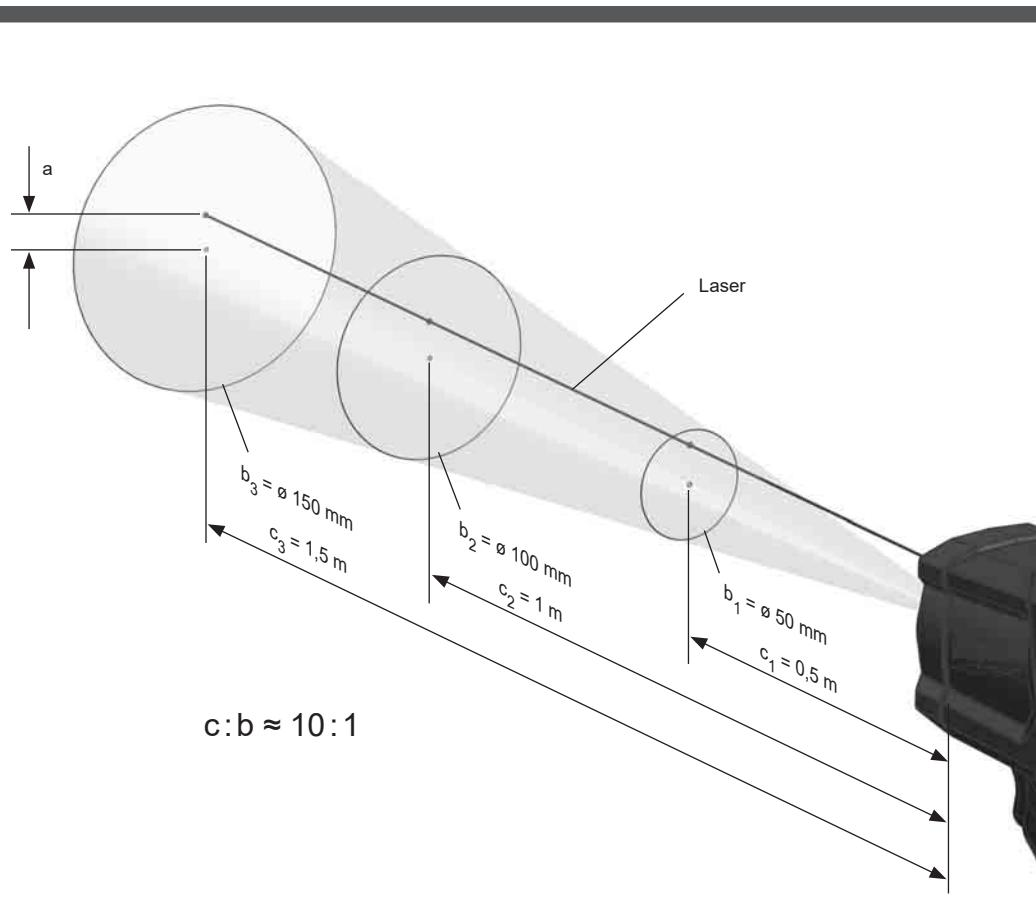
a - Distance laser point to center of spot temperature area (19 mm)
