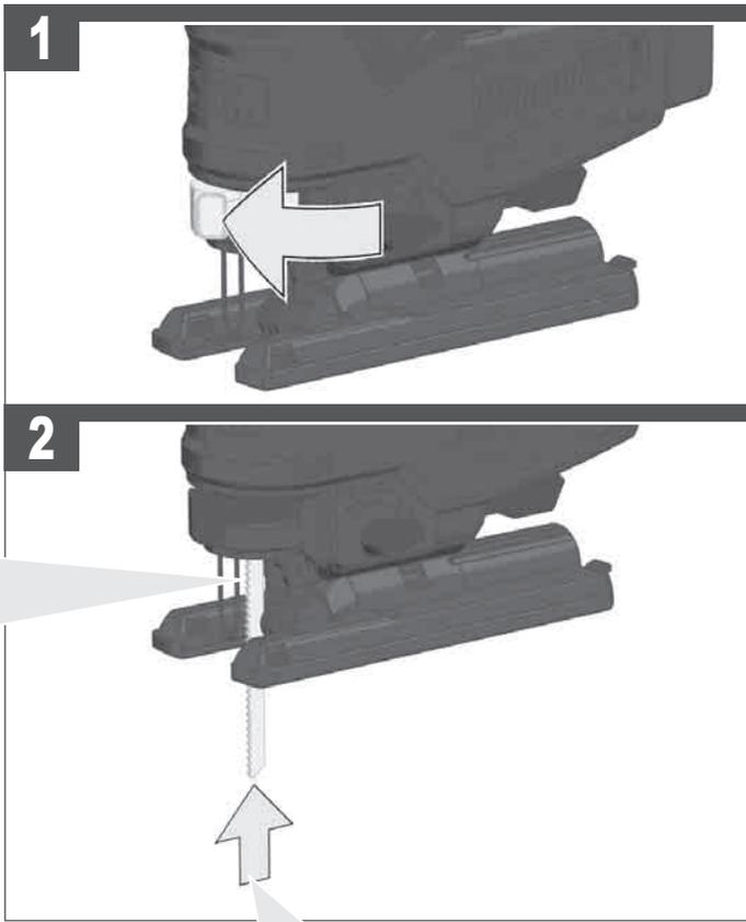
Press the saw blade into the Fixtec holder up to the stop.
