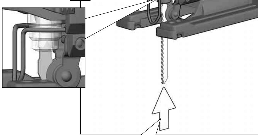
Press the saw blade into the Fixtec holder up to the stop.
