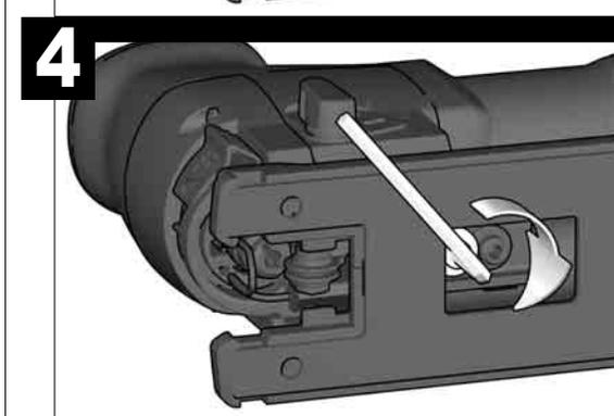
In case the base plate can't be tensioned anymore after frequent adjusting, the base plate setting mechanism can be re-adjusted.
