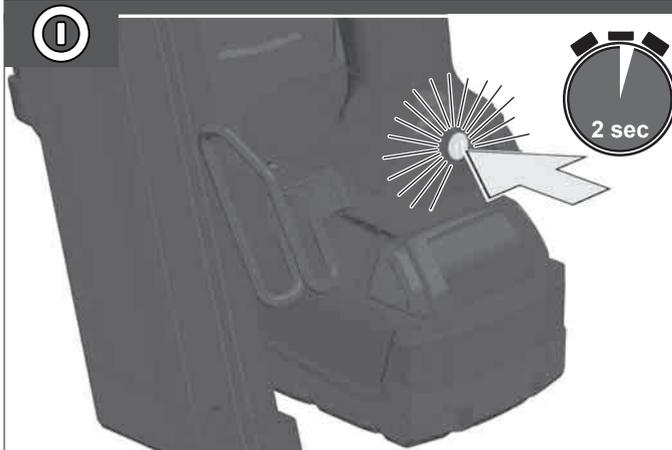
Press and hold the Power/Actuation button to turn on the tool.
