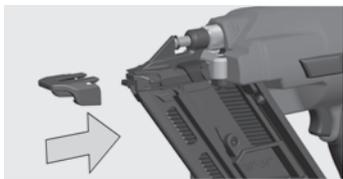
Attach the protective cap to protect sensitive surfaces.
