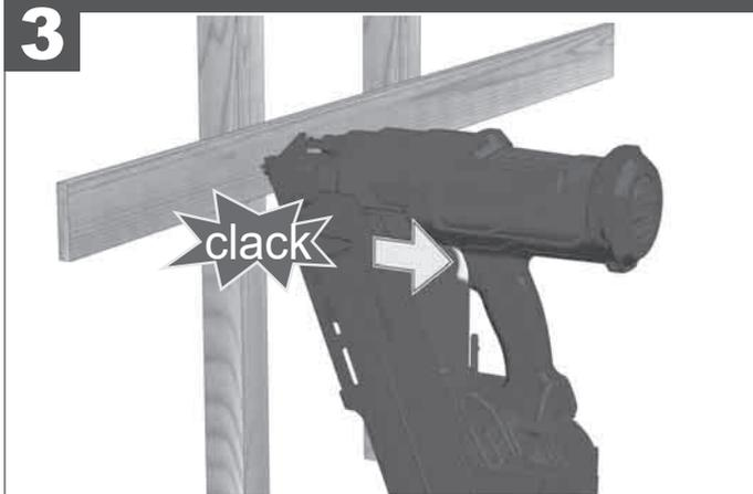
Pull the trigger to drive the fastener.
