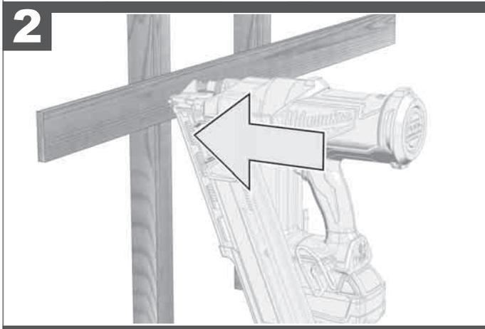
Push the tool against the work surface, compressing the workpiece contact.
