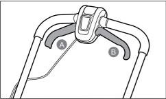
Press the start button and then squeeze the on/off lever (A or B) to start the product. Release the start button and keep squeezing the on/off lever to run the blade. Release the on/off lever to stop the blade.
