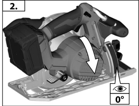
If a correction of the 90° angle of the guide-plate to the saw blade is necessary, use the correction screw.
