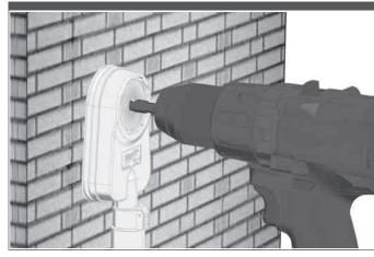
Connect the machine to a suitable dust extractor.
