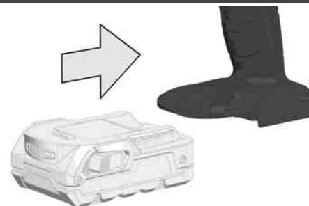
Remove the battery pack before starting any work on the machine.
