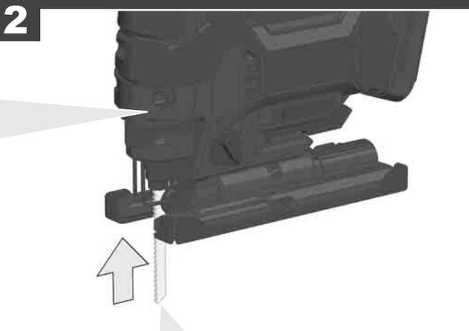
Press the saw blade into the Fixtec holder up to the stop.
