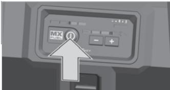
This machine must be activated before switching on.
