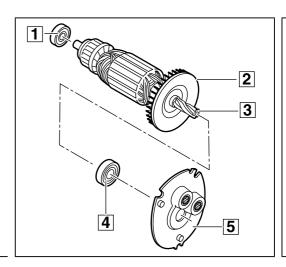
Inserting the armature
