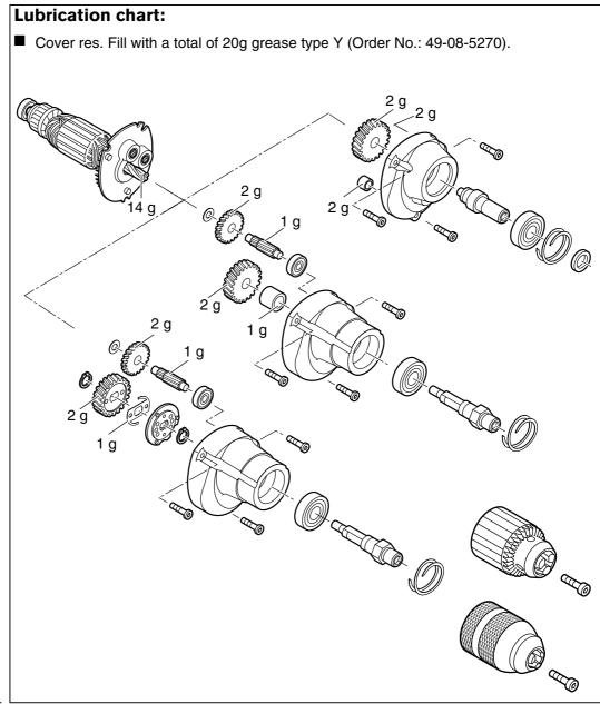
Torques Screws in plastic 1.7 Nm
