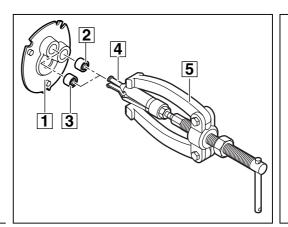
Removing the field and the electronic components
